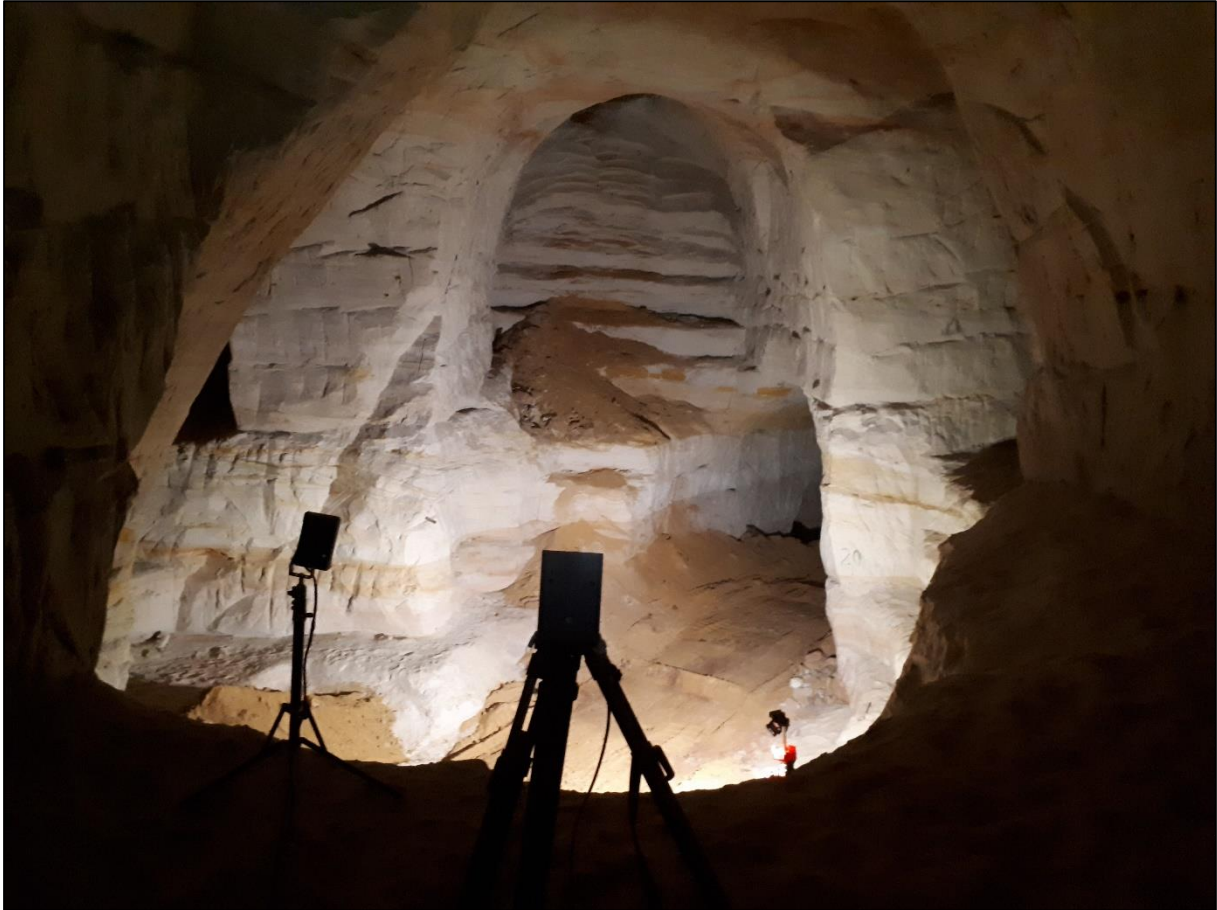
Photo 10. Bat-camera elements installed to the location in Piusa caves where culvert was later installed and then camera gave proof that bats started to fly through the culvert almost immediately after it was installed. At the upper part of the photo can be seen the hole in the ceiling that is a first part of the collapse that we avoided with installing culvert. Photo by Lauri Klein.
